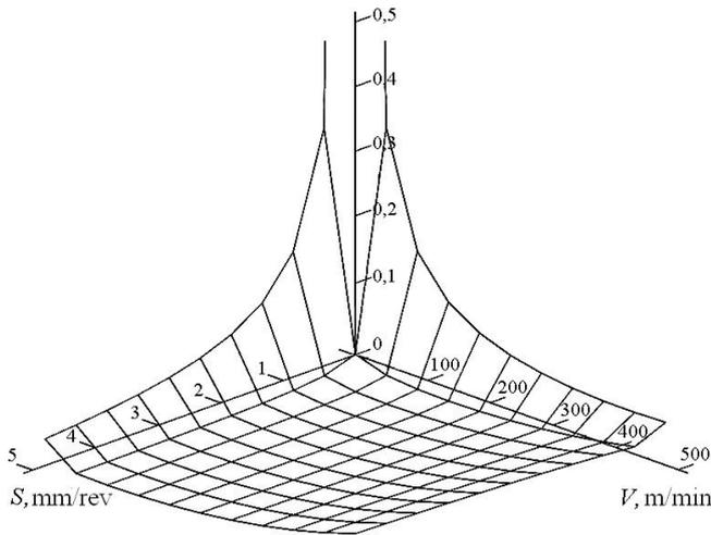
**Fig. 1:** Three-dimensional geometric dependency  $F(S,V)$  model:  $S$  – in-feedings,  $V$  – cutting speed.
