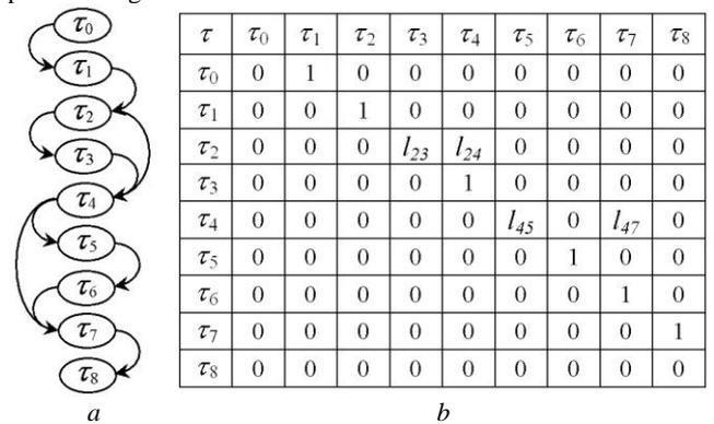
**Fig. 3:** Group technology model:  $a$  is the structure and parameters graph,  $b$  is the adjacency matrix of elements;  $\tau_0 \dots \tau_8$  are technological operations, 0 is falsity, 1 is the truth;  $l_{23}, l_{24}, l_{45}, l_{47}$  are logical expressions.
