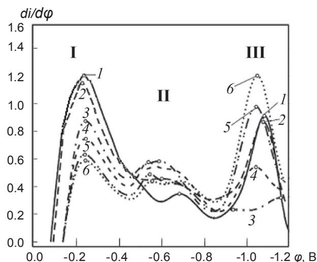
Fig. 5. Differential volt-amperegrams of reduction of free oxygen radicals on a copper cathode against a background of 0.1 M NaCl in water (1) in the presence of various concentrations of GSH ( $T = 298 \text{ K}$ ): 2 – 0.24; 3 – 0.47; 4 – 0.74; 5 – 0.91; 6 –  $1.1 \cdot 10^3 \text{ M/ml}$
