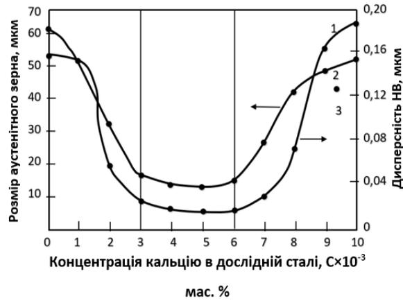
Figure 4 – Influence of calcium concentration on austenitic grain size and dispersion of non-metallic inclusions
