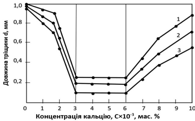
Figure 5 – The effect of calcium concentration on the crack length in the axial section of the sample: 1 - when tested for bending deformation; 2 - axial load; 3 - torsional deformation
