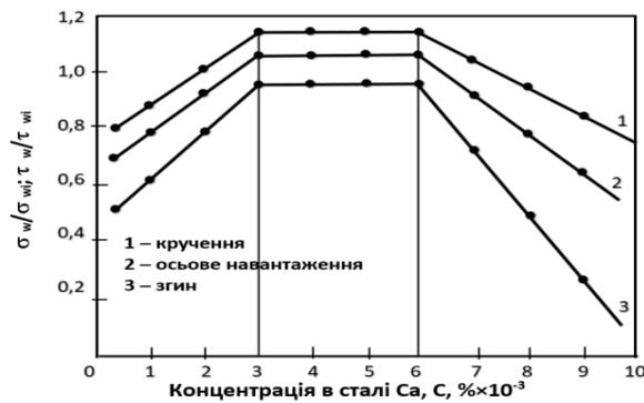
Figure 2 – Fatigue resistance ratio based on  $N = 10^7$  cycles in salt water (5% NaCl) in the torsion test (1), axial load (2) and bending (3)
