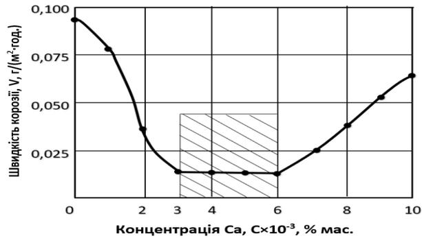
Figure 1 – Influence of calcium concentration on corrosion rate of experimental steel in model aggressive environment: 200 g / l NaCl,  $P_{CO_2} = 1.0$  MPa,  $t = 40$  C. Tests in autoclave installation
