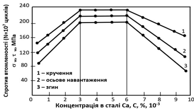
Figure 3 – Relationship between calcium concentration in steel and fatigue resistance based on 107 cycles at torsional deformations (1), axial load (2), and bending (3)
