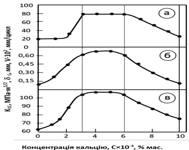
Figure 6 – The effect of calcium concentration in the test steel on the crack growth rate in samples (a), on the coefficients  $dC$  (b) and  $K_{1C}$  (c) when testing samples in air at  $t = -40C$
