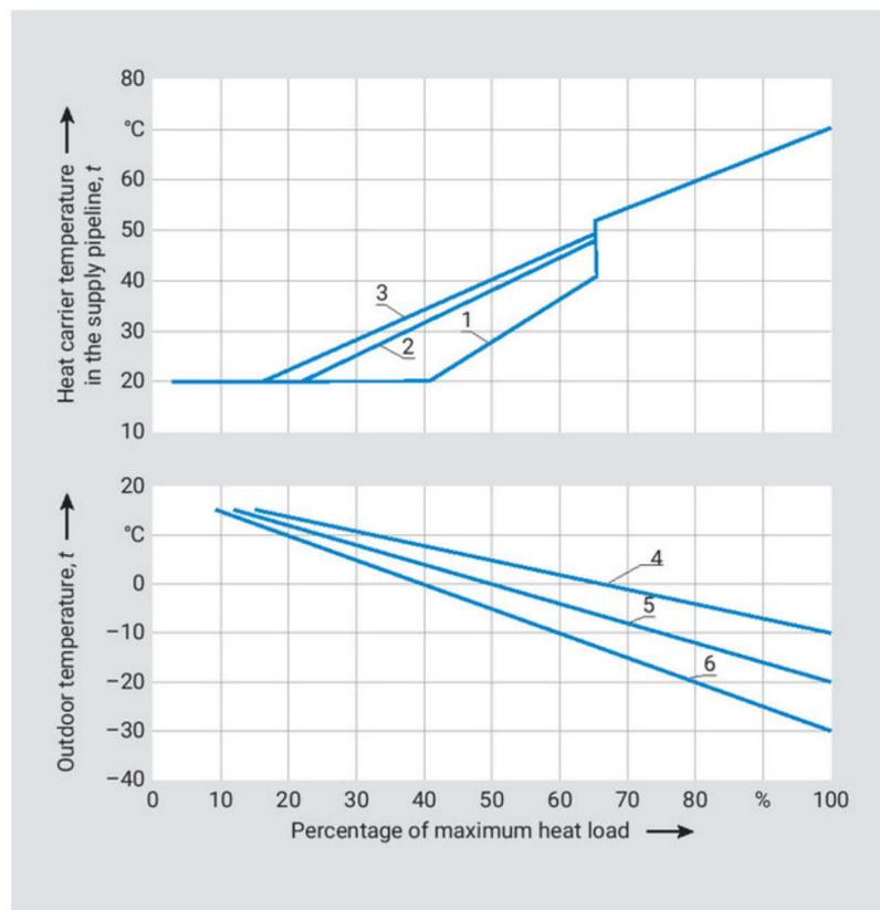
Figure 7. Return temperature for different supply temperatures and different design outdoor temperatures with qualitative-quantitative central control
