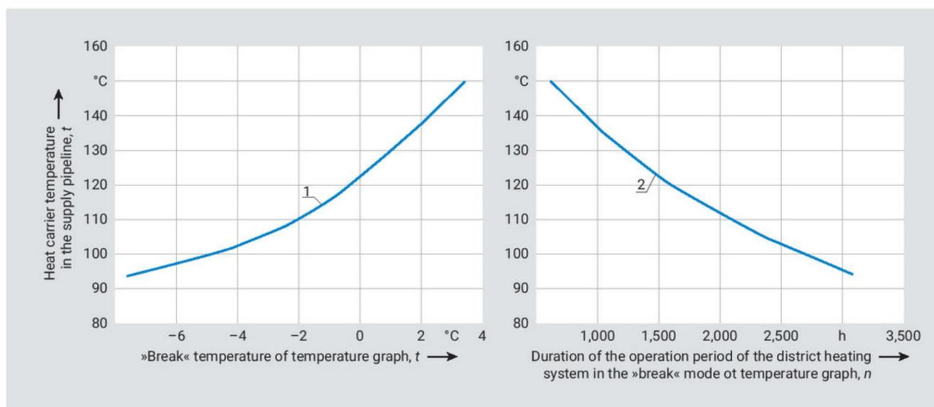
Figure 2. Temperature dependence at the „break“ point and duration of the „overheating“ period on the estimated temperature in the supply pipeline (type of temperature graph) for meteorological conditions in Poltava
