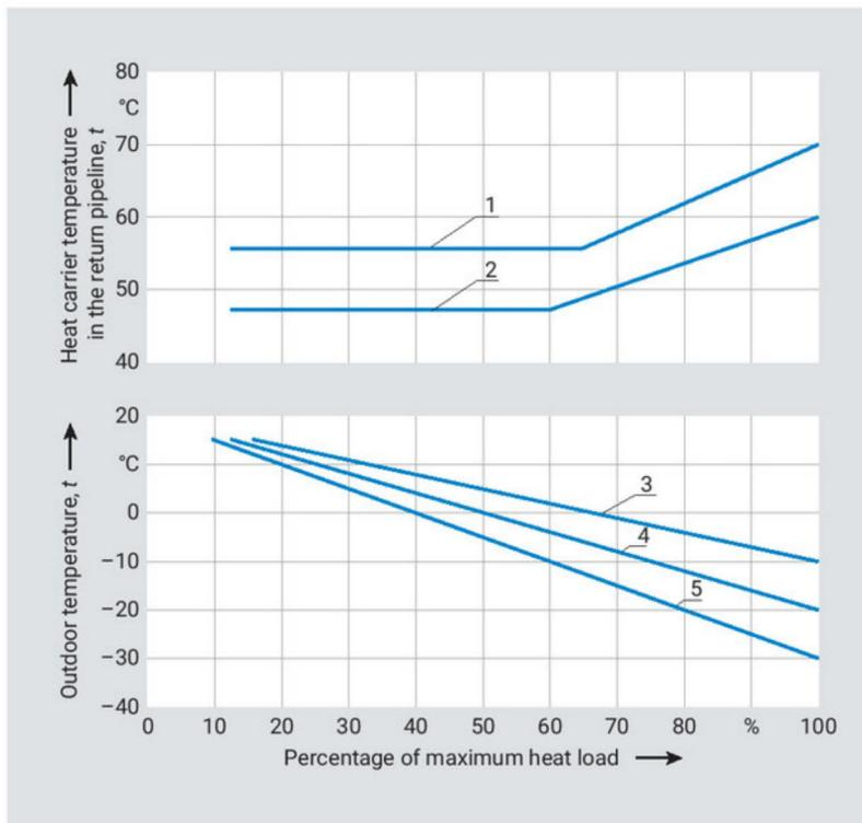
Figure 5. Dependence of the return temperature on different supply temperatures with current qualitative central control
