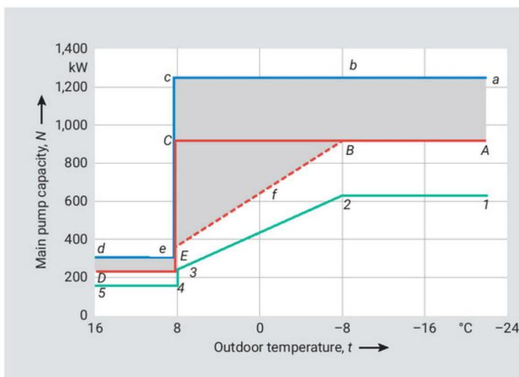
Line a-b-c-e-d: Required capacity of main pumps for the current state of district qualitative control (dependent connection scheme of multi-family buildings, pumps without quantitative control of heat carrier flow)
