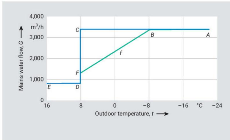
Figure 10. Heat carrier flow change in district heating system depending on the outdoor temperature
