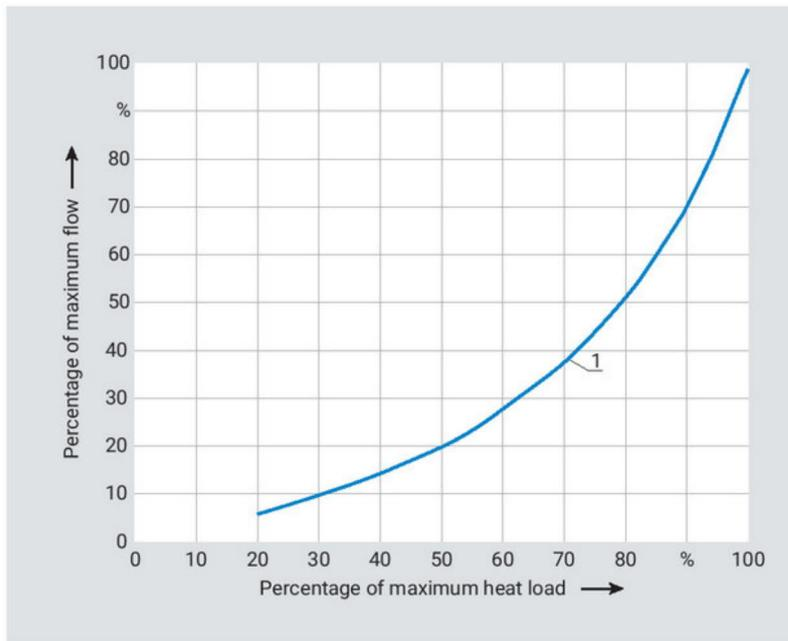
Figure 9. Quantitative central control and determination of relative heat carrier flow for temperature graph 80/60 °C
