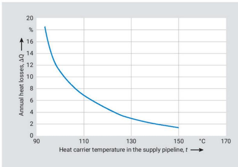
Figure 3. Dependence on annual heat losses  $\Delta Q$  in the “break” mode of the supply temperature for weather conditions of an estimated temperature curve with design outdoor temperature  $-23\text{ }^{\circ}\text{C}$
