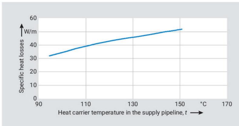
Figure 4. Dependence of specific heat losses on the supply temperature for meteorological conditions in Poltava
