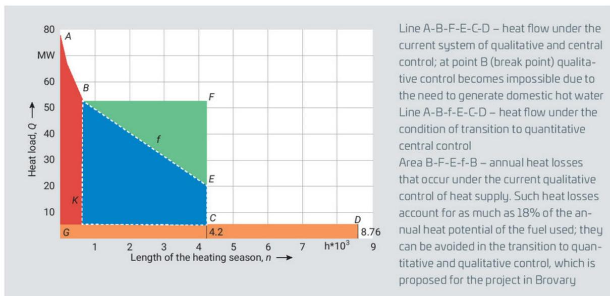
Figure 1. Annual heat generated by boilers in a district heating system for different methods of heat supply control
