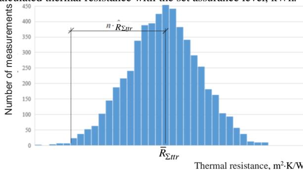
Fig. 1: Histogram of total reduced thermal resistance distribution of the building envelope
