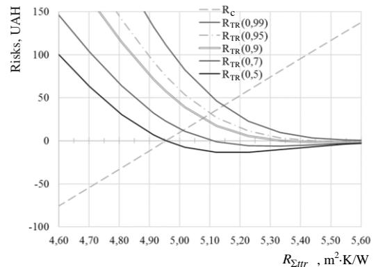
Fig. 5: Dependency graph of the total risks of construction and heating costs on the reduced total thermal resistance (Kyiv, civil building)
