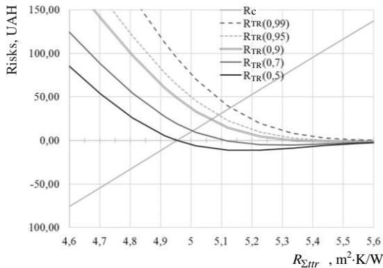
Fig. 3: The dependency diagram of the cost of additional insulation and the risks of additional energy consumption on the reduced total thermal resistance
