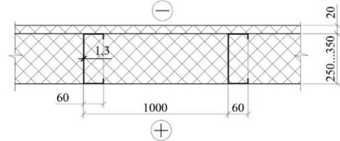
Fig. 2: Structural design of a floor slab structure
