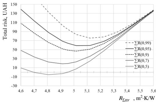
Fig. 4: Dependency graph of the total risks of construction and heating expenses on the reduced total thermal resistance (Poltava, residential building)
