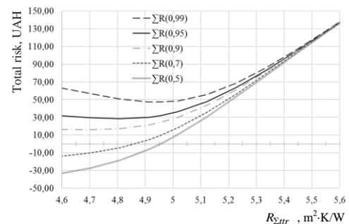
**Fig. 6** : Dependency graph of the total risks of construction and heating expenses for on the reduced total thermal resistance (Poltava, 25 years)
