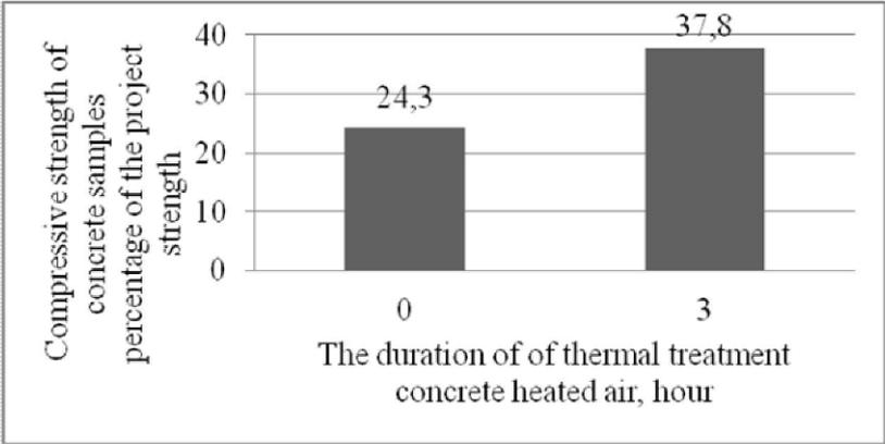
Fig. 5. Compression strength samples with heavy concrete at 2 days, the percentage of design strength (experiment 1)
