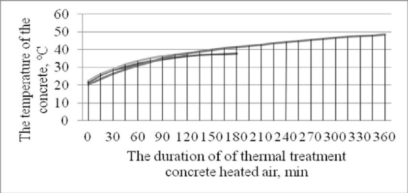
Fig. 4. Changing the temperature of concrete at its heat treatment in heated air solar collector (experiment 1-3)
