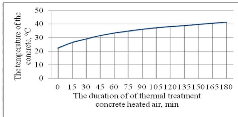
Fig. 2. Changing the temperature of concrete at its heat treatment in heated air solar collector (experiment 2)
