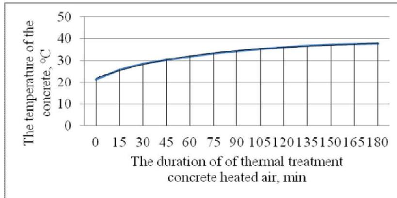
Fig. 1. Changing the temperature of concrete at its heat treatment in heated air solar collector (experiment 1)
