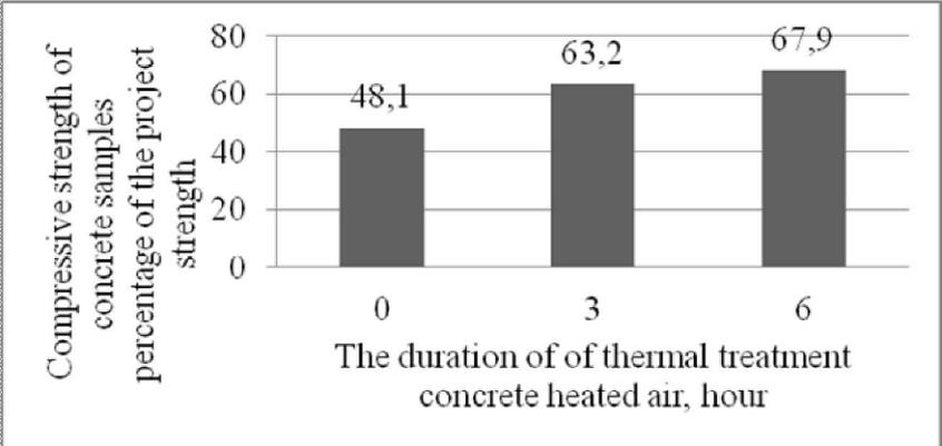
Fig. 6. Compression strength samples with heavy concrete at 5 days, the percentage of design strength (experiment 2, 3)
