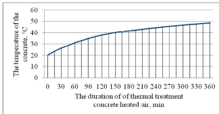
Fig. 3. Changing the temperature of concrete at its heat treatment in heated air solar collector (experiment 3)
