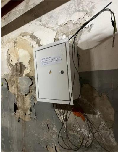
Figure 3 - Mounting the heat flux converter and thermal sensors on the inside of the wall structure
