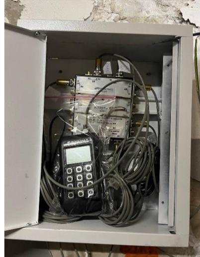
Figure 4 - Measuring and recording complex “Теплограф-4”
