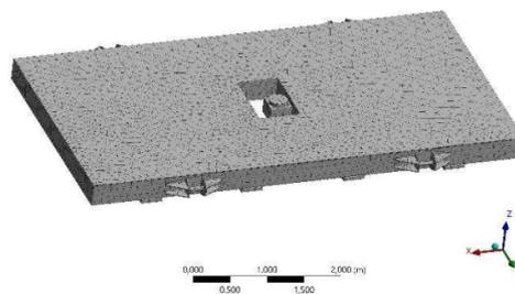
Figure 1 – Design solutions using finite element analysis for the vibration platform
