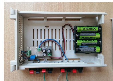
Fig. 3. Analog-to-digital converter with TLC chip:
