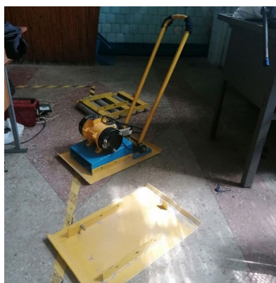
Fig. 6. Vibration plate with replaceable working elements
