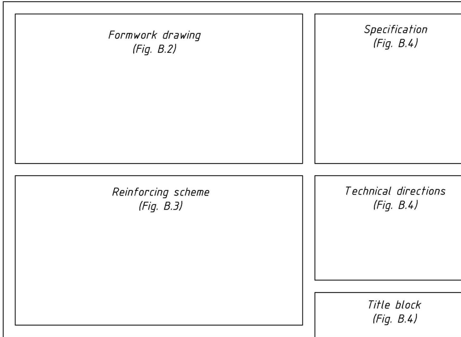
Figure B.1 – Variant of arrangement of drawings of the crane beam on the A2 sheet
