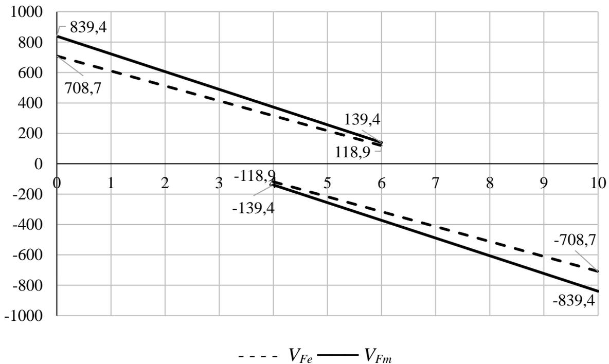
Figure 2.3 – The enveloping shear forces diagrams
