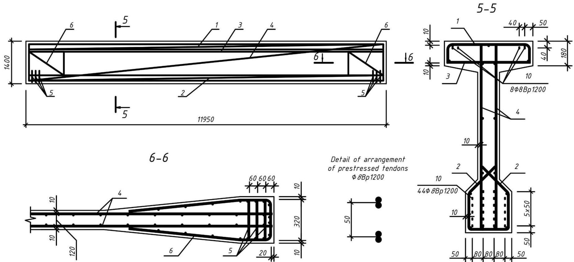
Figure B.3 – Reinforcing scheme
