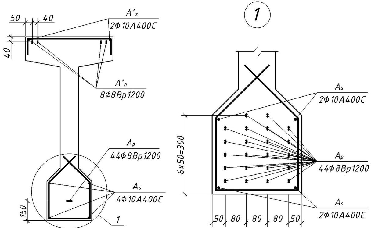
Figure 2.5 – Placement of longitudinal reinforcement
