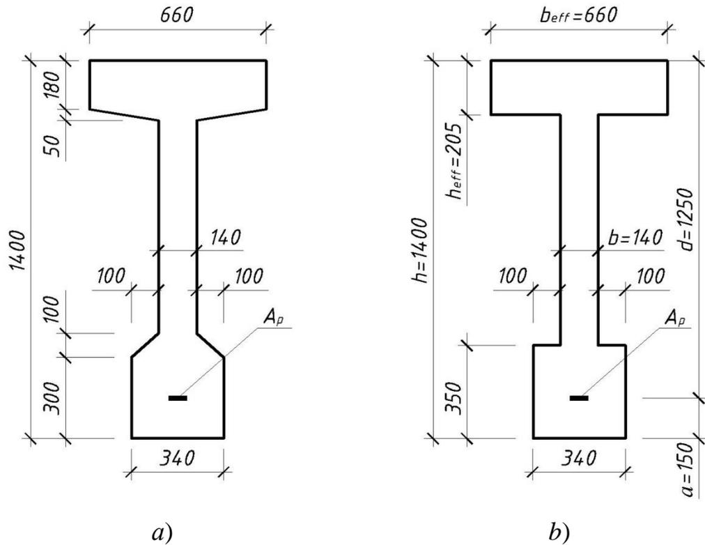
Figure 2.4 – Cross-sectional shape of crane beam section in the span:
