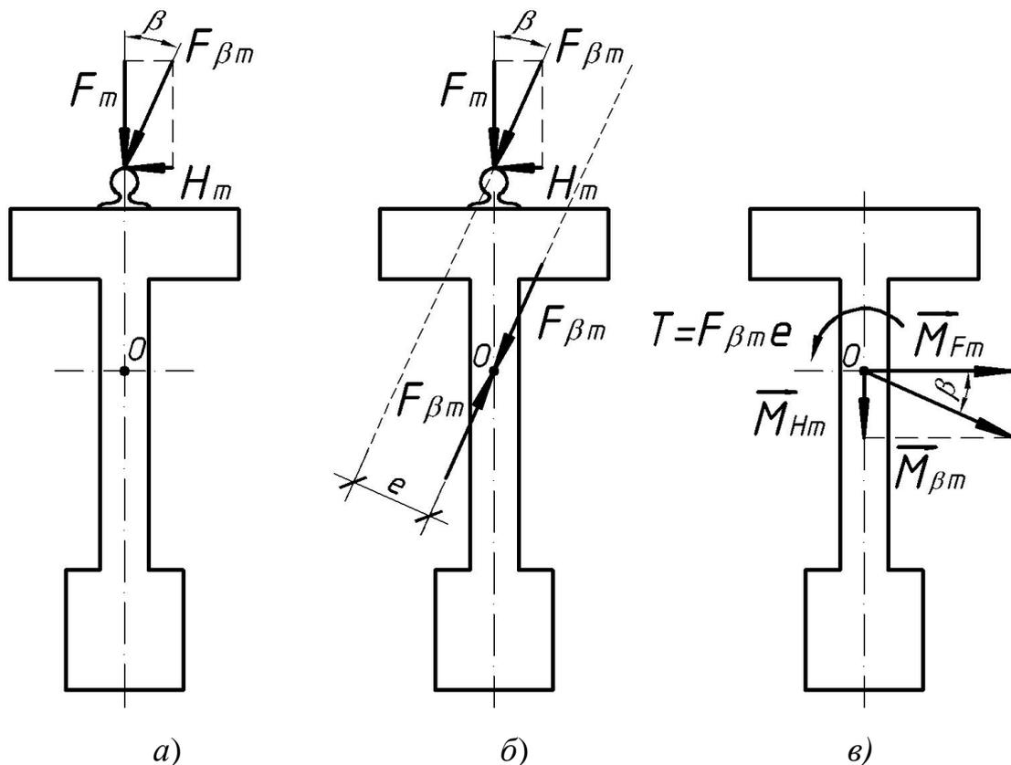
Figure 3.1 – To determination the value of the moment of biaxial bending of the beam: a) scheme of forces; b) scheme of forces in the centre of gravity of the section (O); c) scheme of moment action in the section
