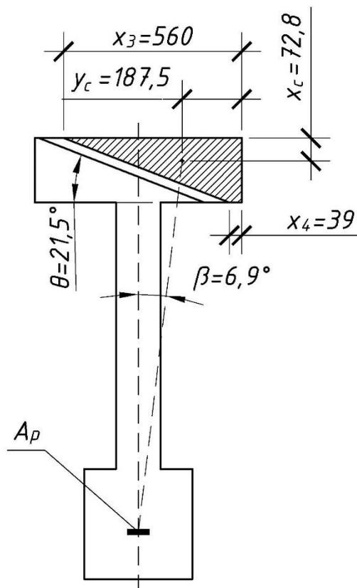
Figure 3.3 – Geometric parameters of the effective compressed concrete area
