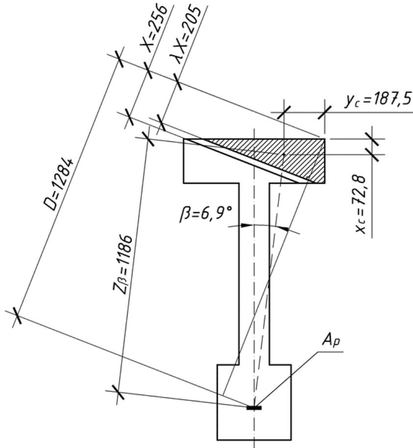
Figure 3.4 – To determination the arm of the internal pair of forces  $Z_\beta$
