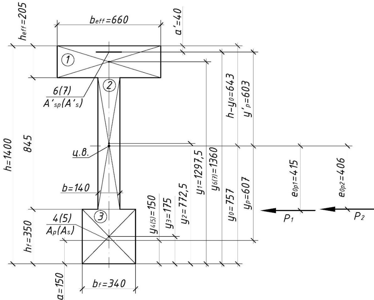
Figure 4.1 – Schematic diagram of the reduced section for the calculation of geometric characteristics and prestressing forces:
