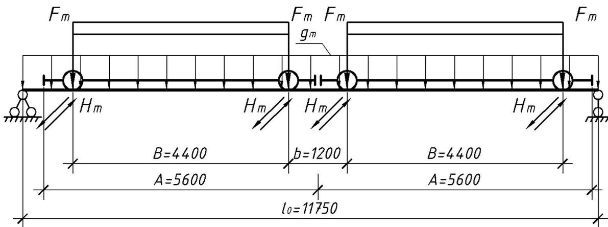
Figure 2.1 – The design scheme of the crane beam for the action of loads from two adjacent cranes
