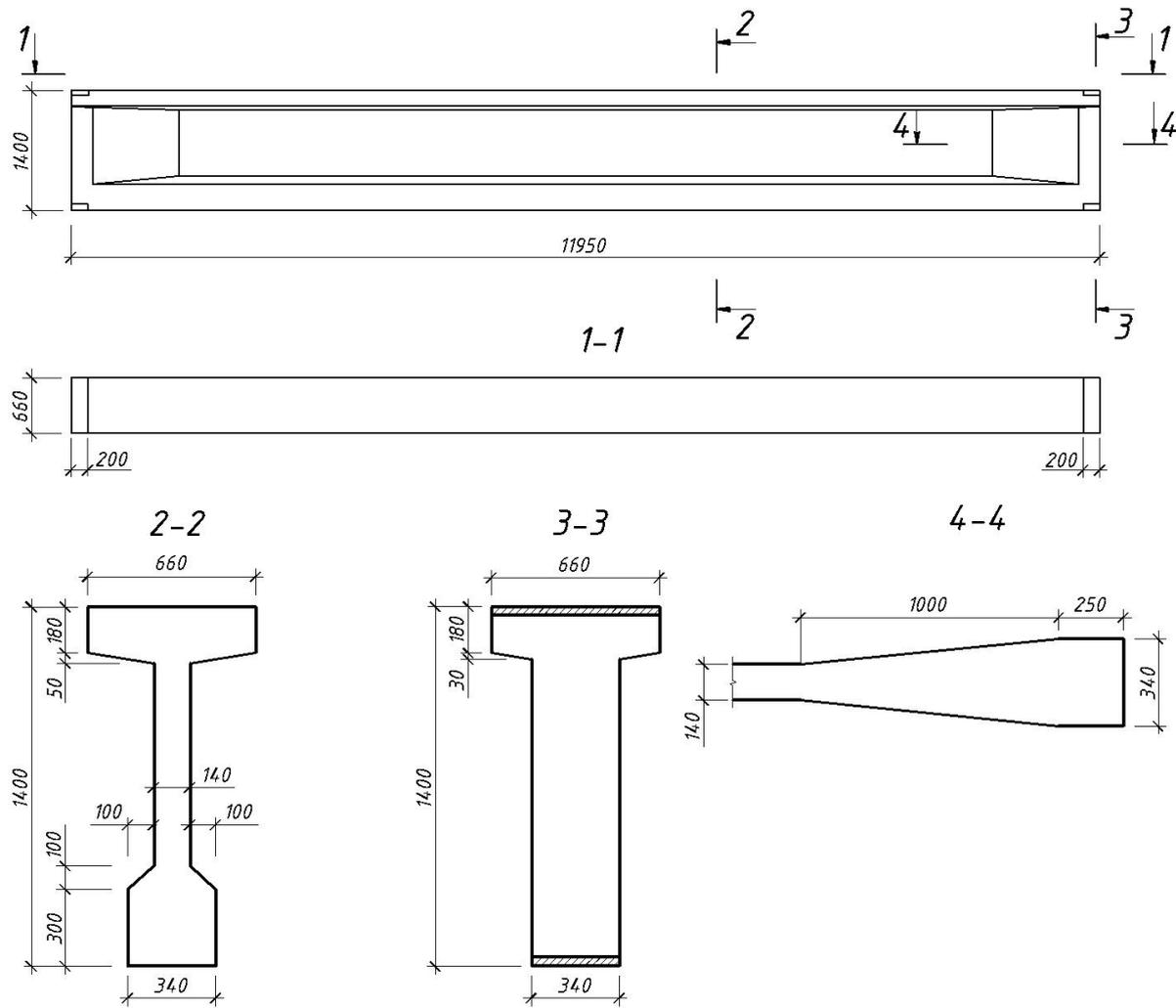
Figure 1.1 – Formwork drawings of the crane beam
