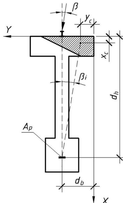
Figure 3.2 – Scheme of the beam cross section to determination the conventional neutral axis position
